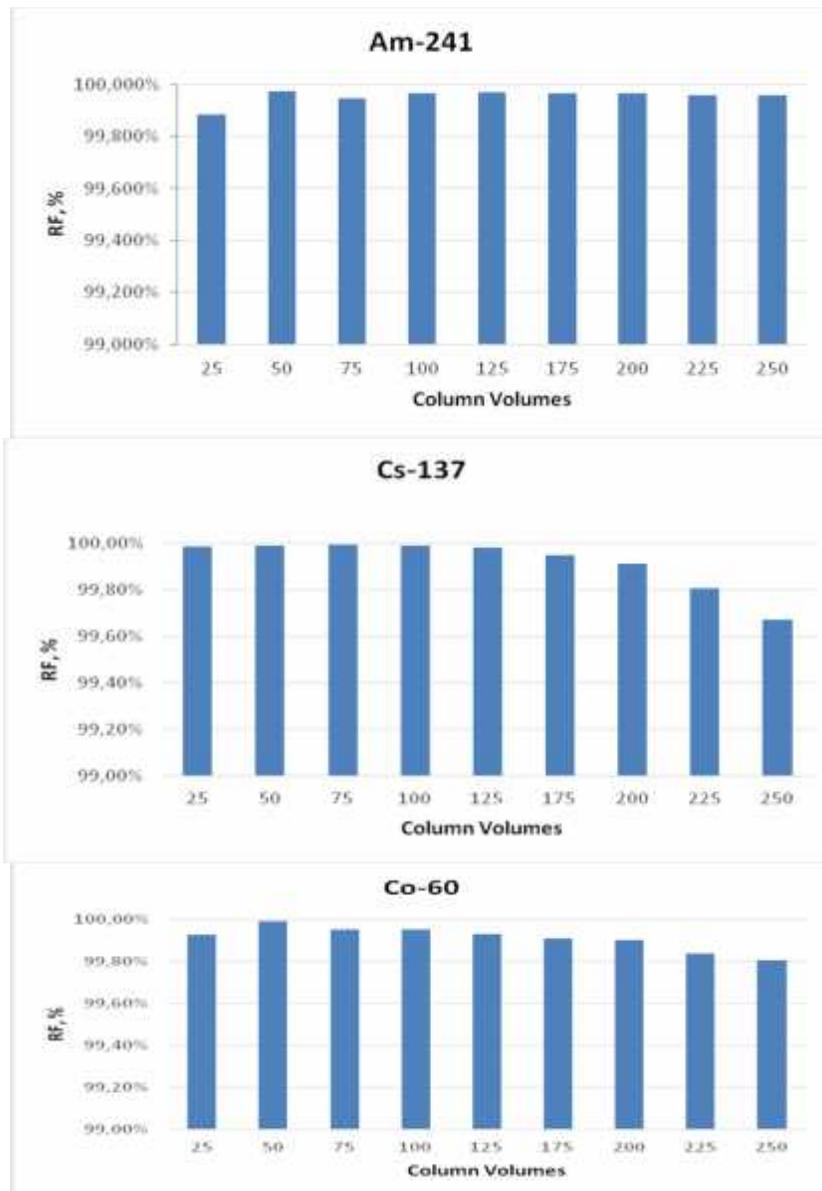
Figure 16. Capacity of Purolite-NRW 1600 with respect to  $^{60}\text{Co}$ ,  $^{137}\text{Cs}$  and  $^{241}\text{Am}$
