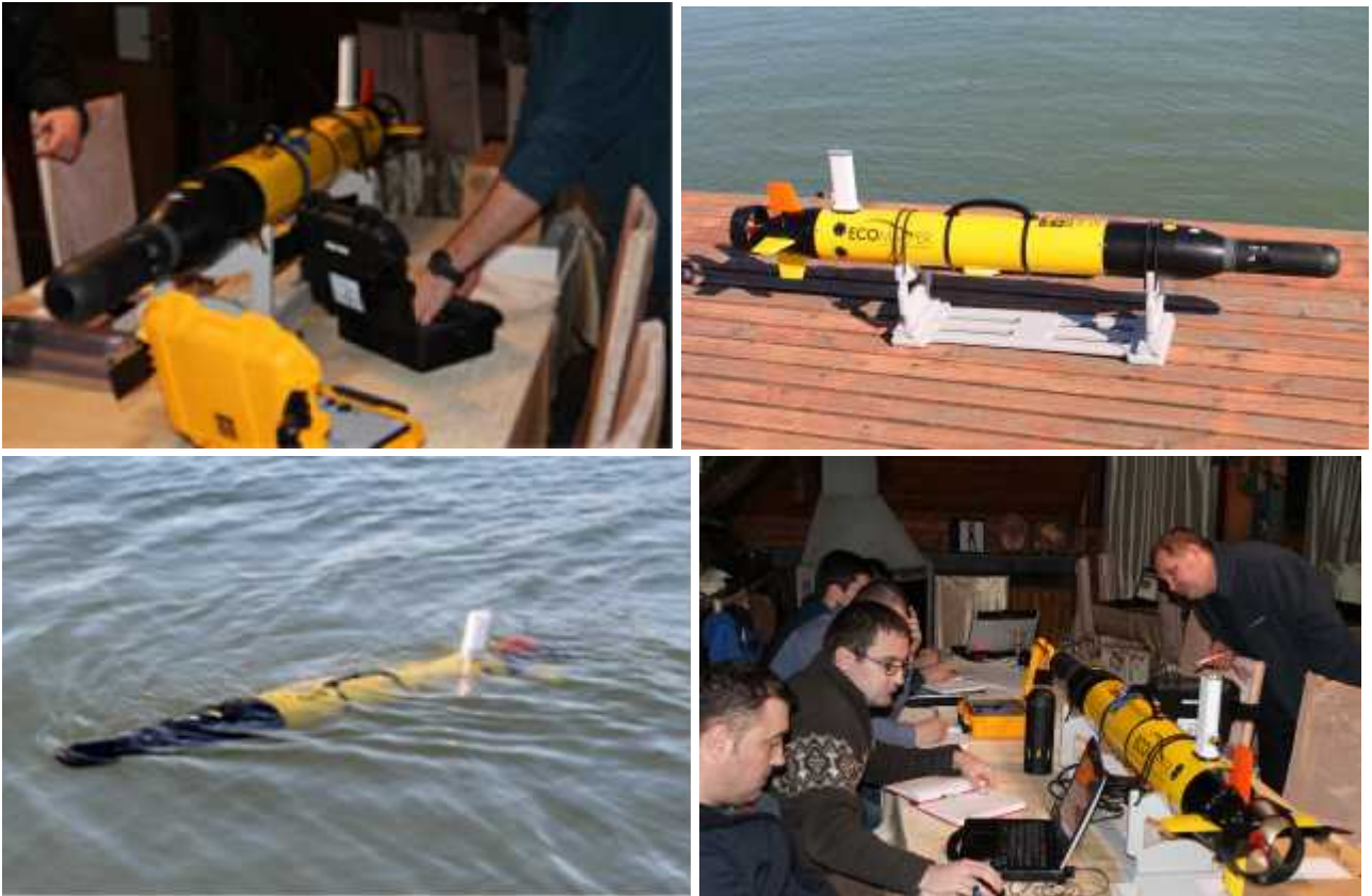
Figure 6. Topo-batrimetry registration equipment (AUV - EcoMapper)
