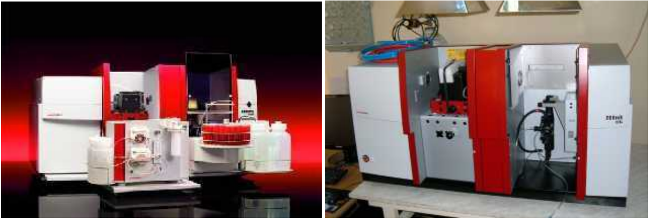
Atomic absorption spectrometer for monitoring heavy metals
