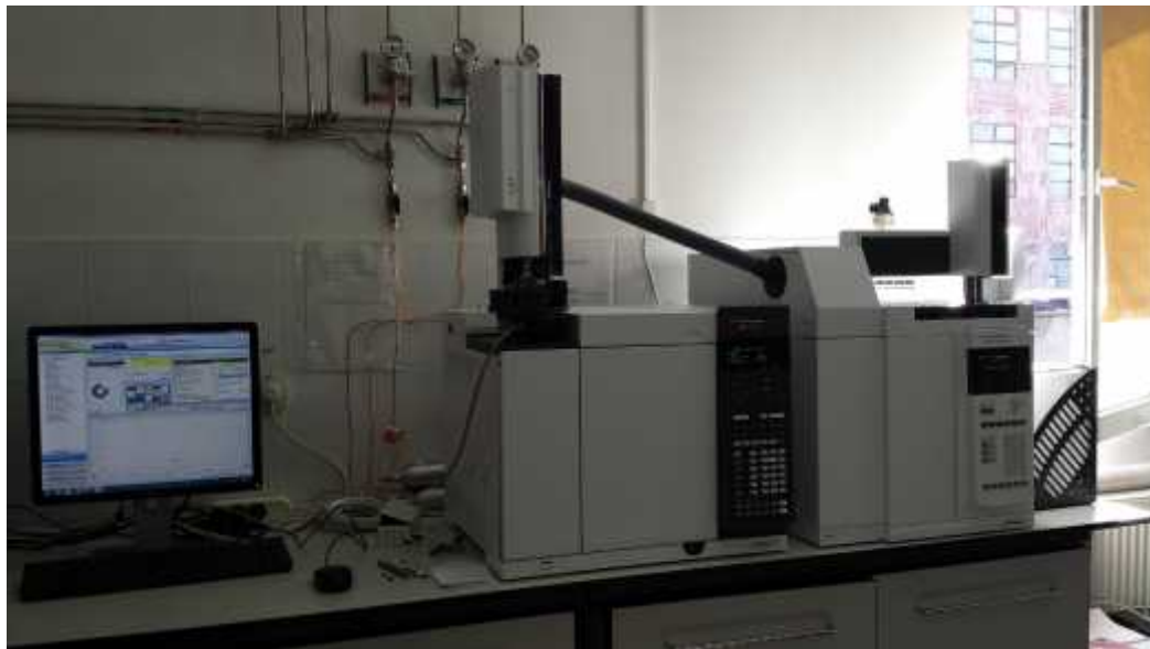
Gas chromatograph for determination of total hydrocarbons and other volatile organic compounds
