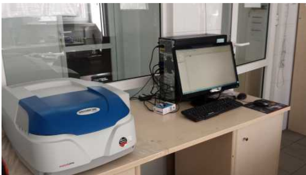
Atomic Absorption Spectrometer for supervision of the main pollutants in water
